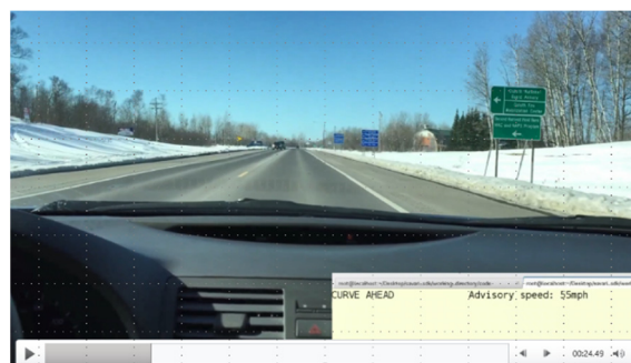
Figure 8: Snapshot from field demonstration showing advanced curve speed warning while approaching a curve.
