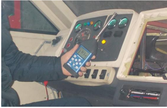
Figure 2: Noise level measured in the cabin of a multi-functional rescue vehicle with a rotary-screw propulsion unit produced by Research and Education Centre “Transport”, Nizhny Novgorod State Technical University n.a. R.E. Alekseev.
