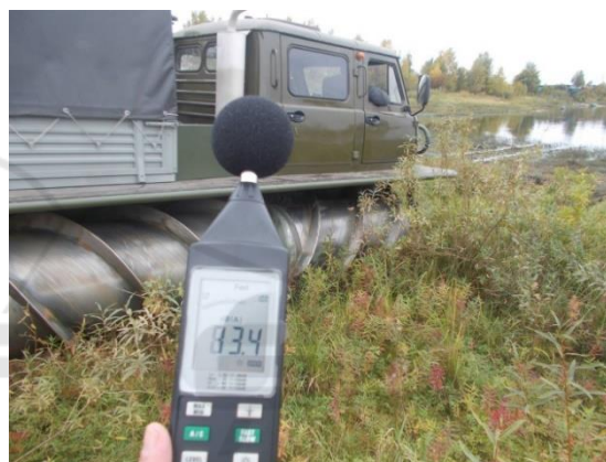
Figure 5: Sound level produced by a rotary-screw propulsion unit on marsh.
