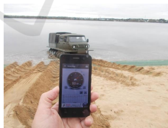
Figure 6: Sound level generated by a rotary-screw propulsion unit on water and sand.
