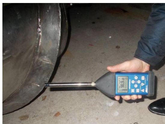
Figure 4: Sound level generated by a rotary-screw propulsion unit on the concrete.
