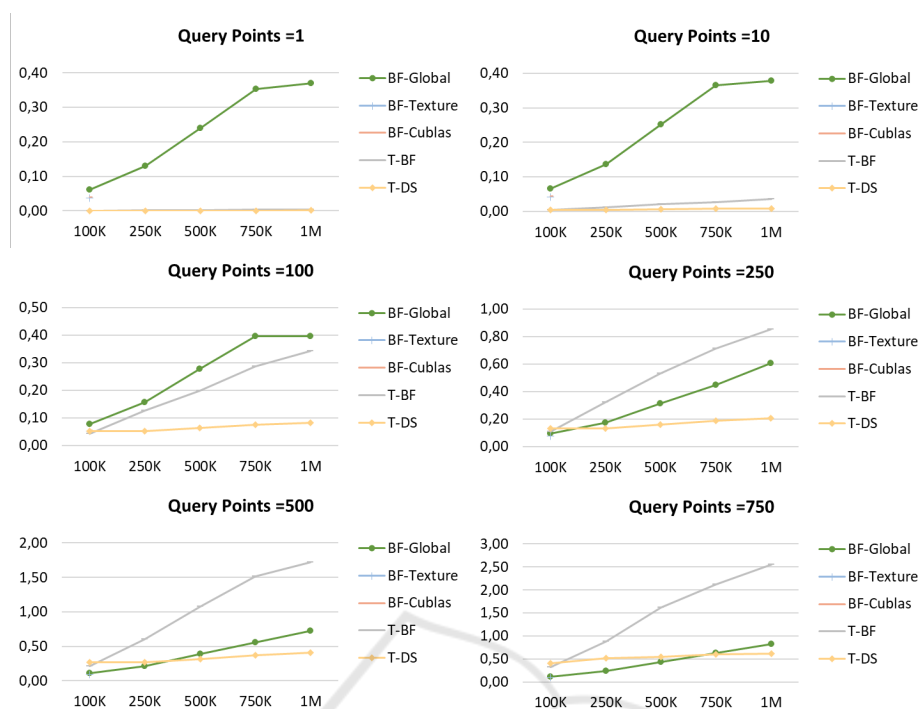
Figure 3: Random reference points, k = 20 . X-axis: reference point cardinality, Y-axis: execution time measured in ms.
