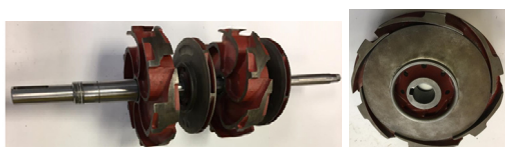
b) Pump stages: impeller and diffuser combined.
