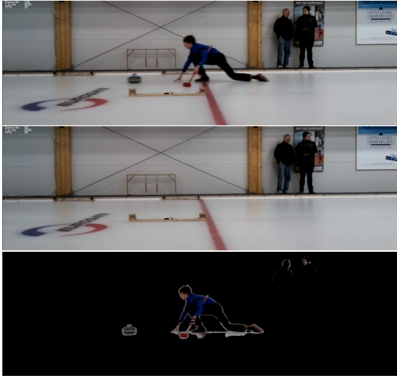
Figure 1: Top: example picture for the background subtraction; mid: reference-Frame used for the background subtraction; bottom: result of the background subtraction.
