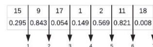
Figure 5: Possible crossover cut points in depth 3; 1 or 1-4 or 2-3 or 3-4 or 4 or 5-6 or 6.
