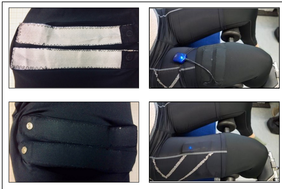
Figure 2: EMG-pants prototype using stainless steel electrodes (top-left). The electrodes are connected via buttons on the outside of the pants (bottom-left) to a sensor module (top-right) by Myon (Myon EMG Mobile System: amplifier, wireless transmission). Standard compression pants were used as a second layer (bottom-right) to improve electrode-skin-contact.
