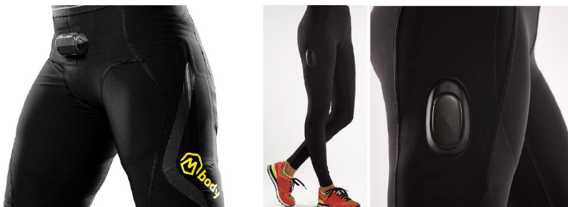
Figure 1: Commercially available spots garments for tracking muscle activity of the thighs by Myontec (left) and Athos (right). Pictures taken from the websites www.myontec.com and shop.liveathos.com on the 21/03/2020.
