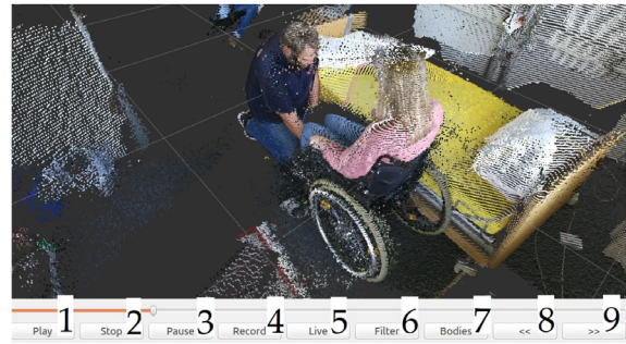
Figure 3: The point cloud player window. Its pixelated appearance is caused by the depth camera resolution of 512 \times 424 . It is possible to play (1), stop (2), pause (3), rewind (8), forward (9) or record (4) point clouds. The live button (5) switches from recording to live data. To reduce the size of the recorded files it is possible to apply voxel grid and statistical outlier filters (6). The coarse body estimation can be turned on, too (7).
