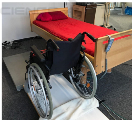
Figure 4: The study setup. A wheelchair is situated beneath a care bed. The transfer is carried out on the force measurement plate in front of the bed.
