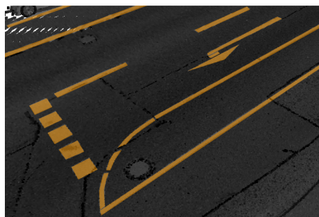
Figure 3: 3D point cloud with detected road markings represented as orange shapes rendered on top of the 3D point cloud.
