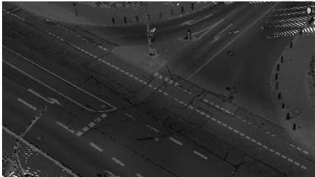
Figure 2: 3D point cloud of a crossing with road markings. Detail of the 3D point cloud shown in Figure 1. Intensity values are represented in grayscale, lighter colors have higher intensity values.
