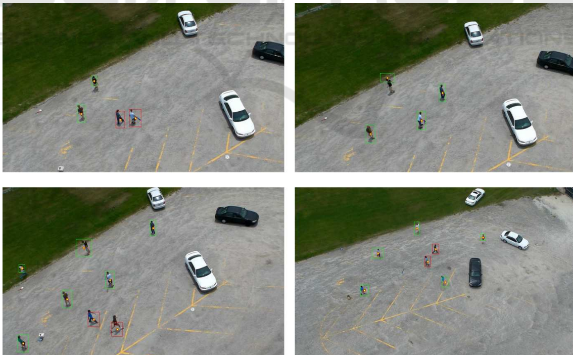
Figure 5: Humans detection, tracking and social distance monitoring samples using the proposed macroscopic method on the UCF-ARG dataset (Nagendran et al., 2010).
