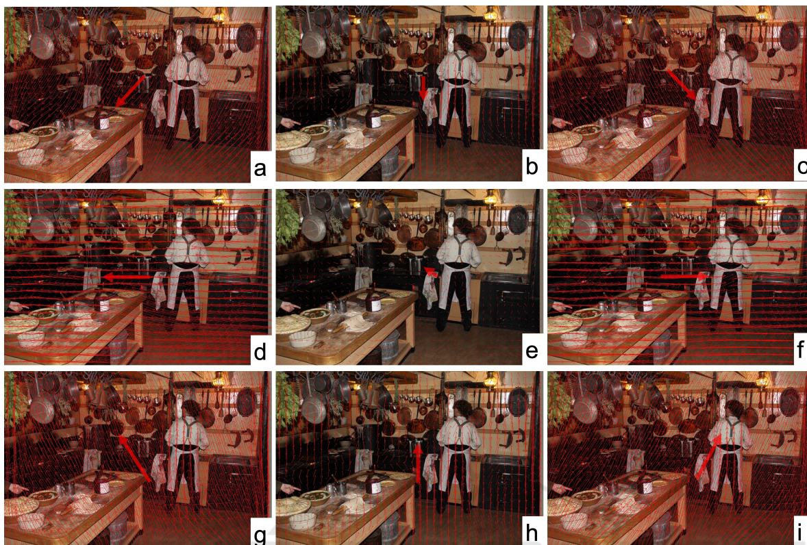
Figure 1: The offset fields for 3 \times 3 kernel points for a deformable convolution with respect to an example image in the validation dataset from COCO. The small arrows in (a)-(i) represent the offset field for each kernel point and the thick arrows in central show the trends of offset for each kernel point.
