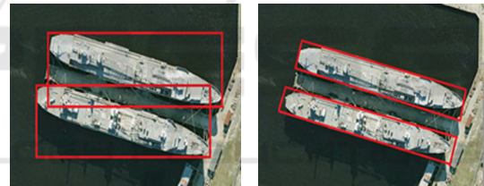
(a) Horizontal bounding box (b) Oriented bounding box
