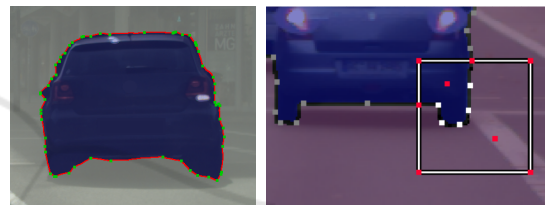
Figure 5: (left): Visualization of the estimated annotation clicks obtained by the RDP algorithm applied to the segmentation contours of a predicted segment of class “car”. The segment contours are highlighted by red color, the obtained vertices (estimated clicks) are highlighted green. (right): Example of possible types of clicks we can take into account for a cost definition. The white (and gray) pixels depict true annotation clicks obtained from the data of (here 5 polygon clicks within the box). The red ones represent additional types of clicks: the ones required for annotating intersection points of segment contour and box edges (here 2 intersection clicks), the ones for defining the box itself (4 box clicks, one for each corner) and one click per segment to specify the class of the segment (here 2 class clicks: for car and street).
