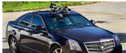
Figure 2: Forward stereoscopic vision system mounted on rooftop of the RoadLAB experimental vehicle.
