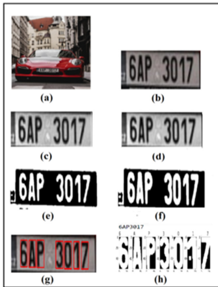
Figure 2: License Plate and Character Recognition in different scenarios. (a) Vehicle, (b) Detected Plate, (c) Gray LP, (d) Blur LP, (e) Binary LP, (f) Dilation LP, (g)Character detection, (h) Digit Recognition.
