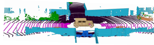
Figure 8: Point cloud segmented by LatticeNet (Rosu et al., 2020) and visualized with the colormap of SemanticKITTI (Behley et al., 2019).
