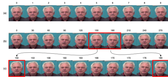
Figure 2: Frame selection methods: (a) First-10 (b) Equal Interval (c) Most Changes: ten frames extracted between frame 150 and frame 180 having the least similarity score.
