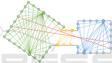
Figure 2: A set of sample points O (convex clusters in green, orange and blue) with exemplary line-of-sights LoS(O) for each convex cluster (framed circles) of the input model. Red lines show inter-partition line-of-sights and grey lines correspond to a piece-wise linear approximation of the surface inferred from the samples. Within a convex cluster, the line-of-sights form a fully connected graph with the cluster samples as nodes. Note that when two mutually visible points belong to the same plane, we do not draw the corresponding line-of-sight for illustration purpose.
