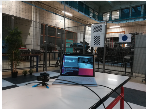
Figure 1: The environment setup of the system: event-based camera, checkerboards, VICON system.
