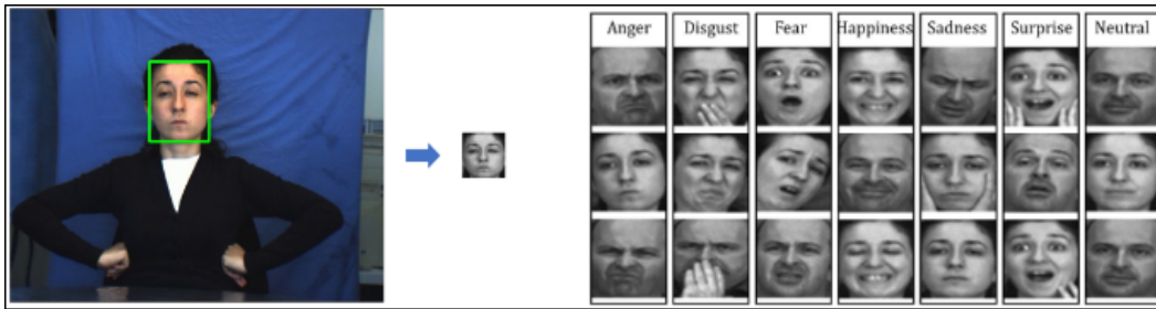
Figure 2: Selection of the facial region on a frame from the FABO dataset and scaling into 48*48 to form image database.
