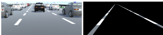
Figure 7: Camera images of the vehicle. Left: Camera for input images. Right: Camera for output images (only lane markings).
