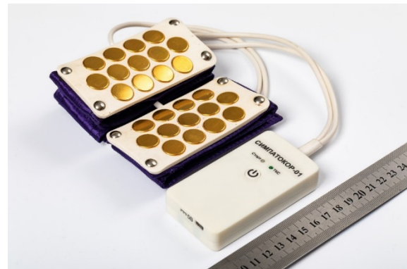
Figure 3: General view of the first module of polyfactorial electrostimulation device.
