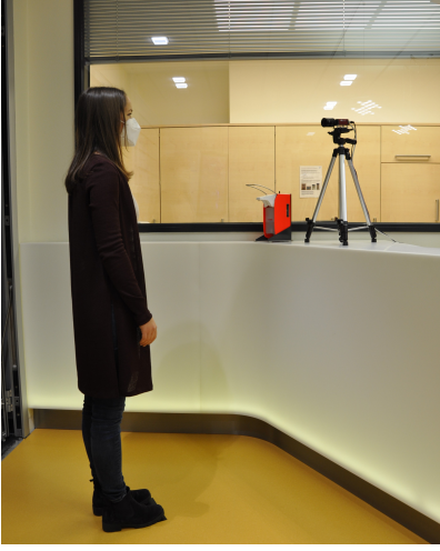
Figure 1: The proposed system for contactlessly measuring the respiratory rate in a hospital-like environment. The camera can be located 1.5 m away from the subject and the evaluation can be done in a safe distance or behind a glass panel by medical personnel.
