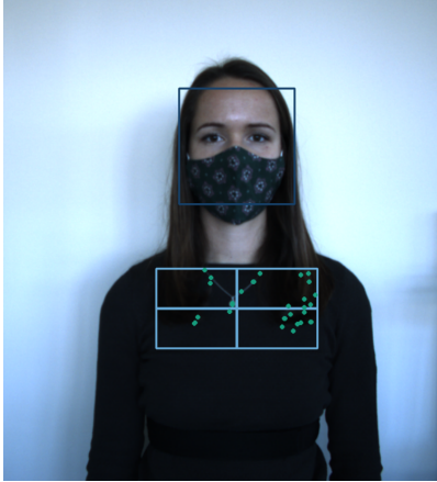
Figure 3: The face is detected to set the position of the ROI relatively to the position and size of the face in the image. Subsequently the ROI is divided into four subregions in which the strongest features are identified and tracked.
