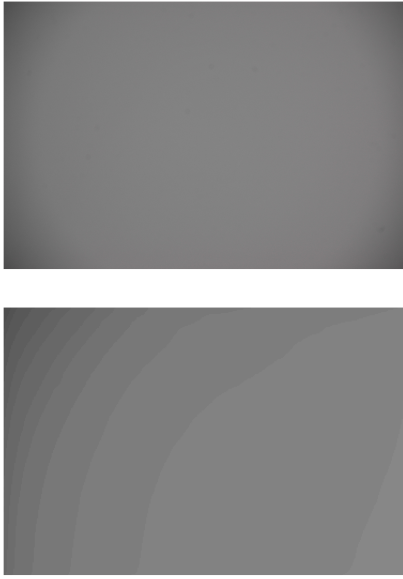
Figure 2: Two different PRNU representations: Top: Conventional PRNU matrix, Bottom: PRNU matrix whose values have been sorted row-wise and then column-wise.
