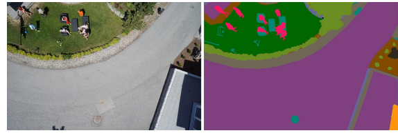
Figure 5: Sample image (left) and the corresponding annotation (right) from the ‘Semantic Drone Dataset’ (Graz University of Technology, 2020).
