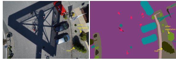
Figure 6: Example image (left) and the corresponding annotation (right) from the ‘Semantic Drone Dataset’ showing high inter-class similarity between the classes ‘tree’ and ‘other-vegetation’. Best viewed when zoomed in.
