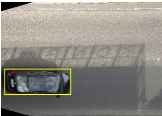
Figure 5: Visualization of the size estimation for the infrastructure-based system. A vehicle entering the recorded area is shown. The estimated size is visualized as yellow bounding box.
