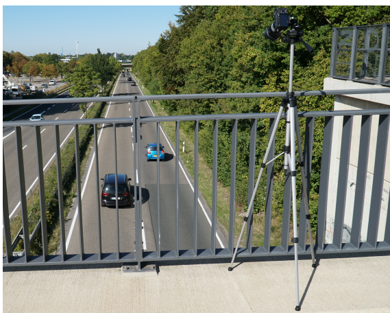
Figure 2: Photo of the recording setup. The camera is positioned on a tripod on a bridge and records the passing traffic from behind.
