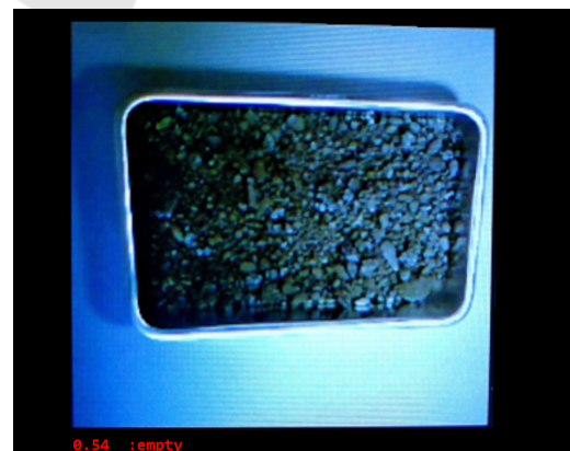
Figure 9: Example of error in recognizing quasi-particles simulating sampling in an industrial environment during the test using SiPEED.
