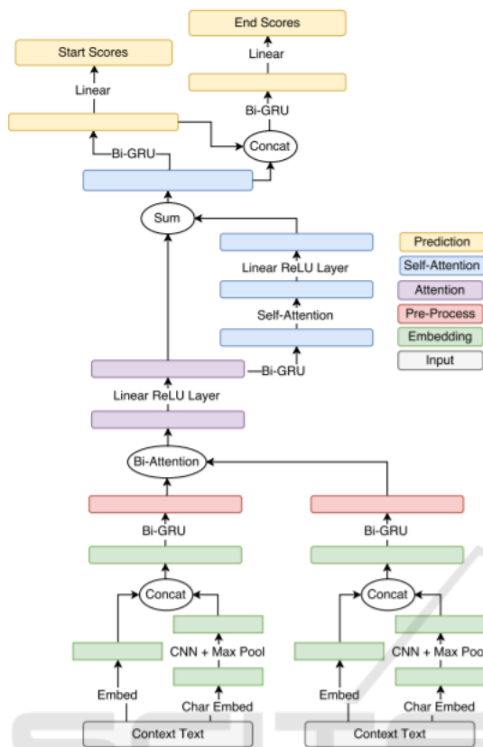
Figure 3: Multi-Paragraph Reading Comprehension architecture; figure courtesy of (Clark and Gardner, 2017).
