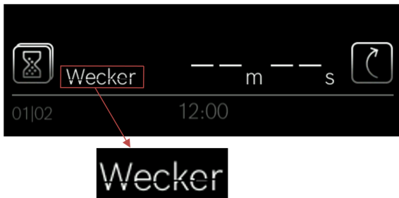
Figure 1: Example of a pixel error of an user interface. The word “Wecker” contains pixel errors as some of the white pixels are missing.
