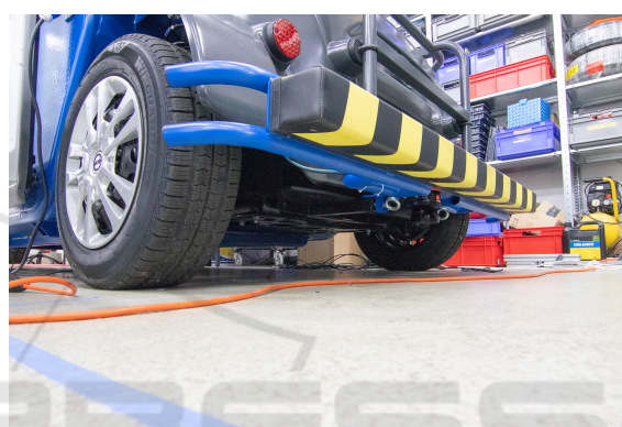
Figure 7: The safety bumper is shown in yellow and black strip. Bumper placement for safe stop is place at the front and rear.
