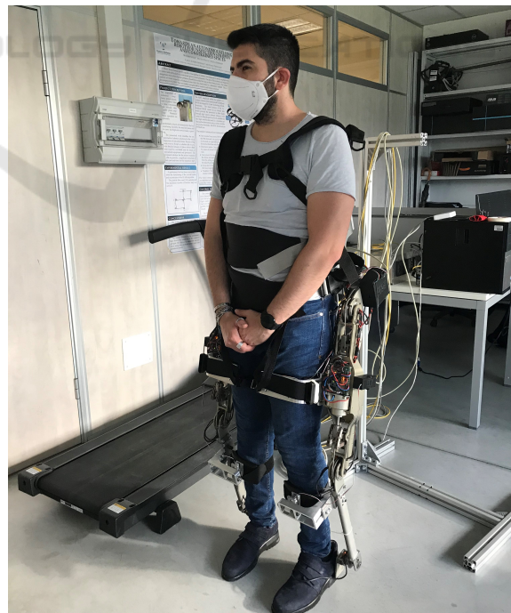
Figure 1: The Wearable Walker lower limb exoskeleton and the experimental setup used for data collection.
