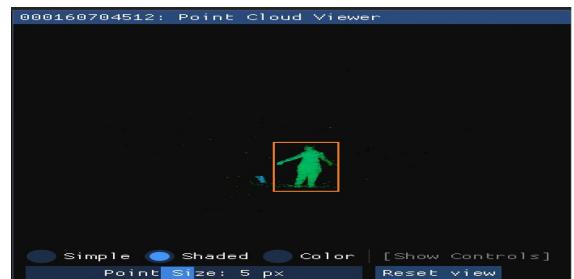
Figure 3.1.4: Human detection by VoxelNet approach from the Azure Kinect Point Cloud.
