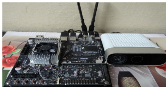
Figure 2.2.1: Edge AI Setup Leveraging Azure Kinect DK Accelerated with NVIDIA Jetson Tx2.
