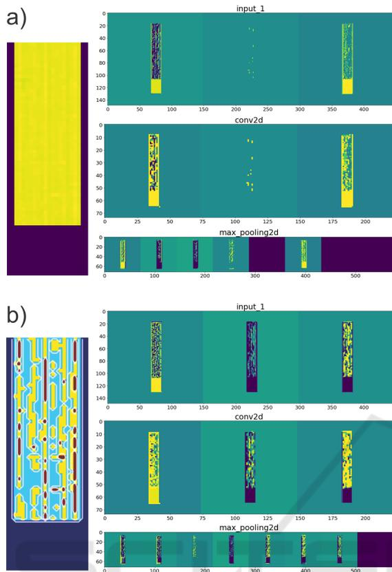
Figure 7: The three initial layers output analysis of using different types of images as input to train/test algorithm. a) Optical Density (OD) profile values of metalized film used as objects and the respective initial layers outputs. b) OD profile films after semantic segmentation with four OD regions classes representation used as input to train/test algorithm and his respective initial layers outputs.
