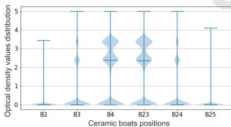
Figure 4: Optical density data set description for local coating systems with his values description according to the position of the sensors. The optical density distribution demonstrate that some positions presents a lack of valid values that should not be considered.
