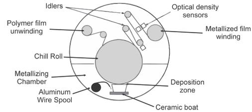
Figure 2: Vacuum Metallization process illustration. Where the polymer film is fed and metallized through vacuum metal deposition.
