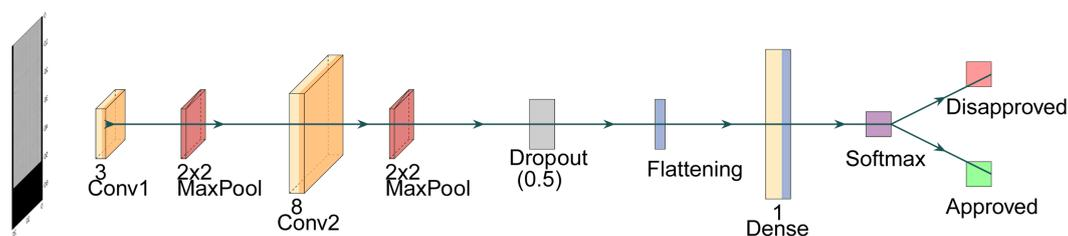
Figure 3: Deep Neural Network used to film class prediction obtained through sequential models from Keras API. We can observe two convolutional and max-pooling layers in the model that extract information, followed by the dropout regularization to avoid over-fitting and, at last, a softmax activation function for final classification.
