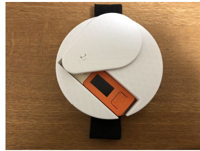
Figure 7: AroNap module with built-in various sensors and aroma stones.
