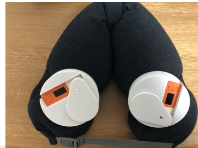
Figure 8: AroNap module attached to the neck pillow.
