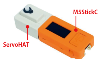
Figure 4: M5StickC and ServoHAT connected.
