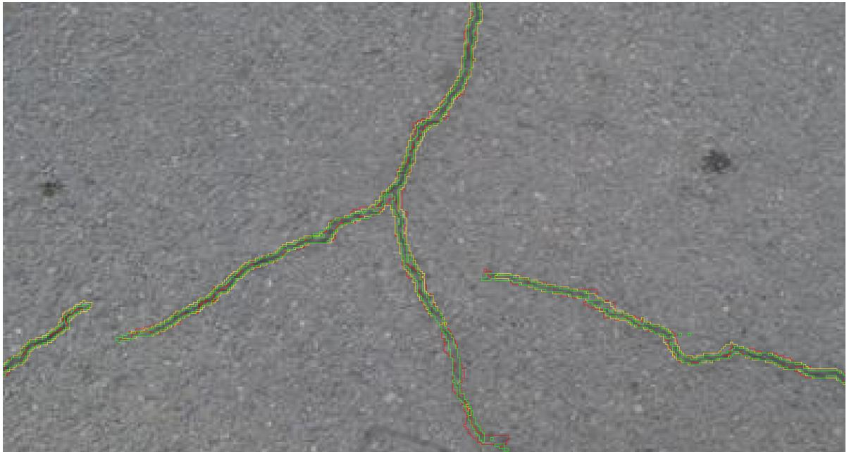
Figure 13: A close-up detailed view of the picture depicted in Fig. 12. The red line is the border of the manual annotation, the yellow line is the border of the prediction obtained by training on CFD, and the green line is the border of the prediction obtained by training on Syncrack hard.
