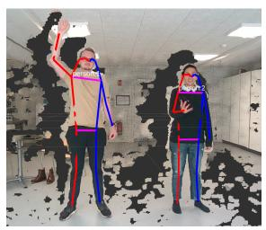
Figure 3: Visualization of the detection and tracking system on people doing the *Get Attention* and *Come Here* action. 2D pose estimations are projected to 3D using the available depth data and the people are assigned a unique ID using the tracker. The 3D poses and ID's are visualized together with the point cloud.
