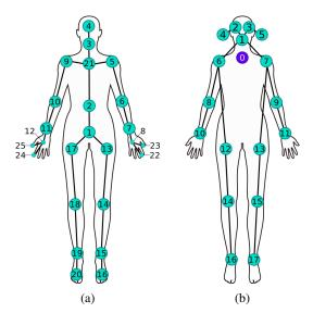
Figure 2: The skeleton models used in the (a) NTU RGB+D and (b) COCO datasets.
