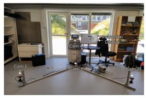
Figure 4: Recording setup. A display instructs the subject which gesture to perform to the robot. This is recorded with four different cameras.
