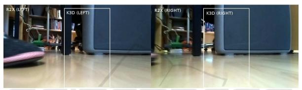
Figure 2: FOV comparison between robot R2X and K3D.
