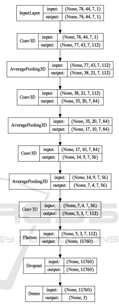
Figure 3: Final disparity-sensitive model NCC-DISP for R2X and OUT. The K3D model was slightly smaller since its input was only [62,48,7,1] but was otherwise the same.
