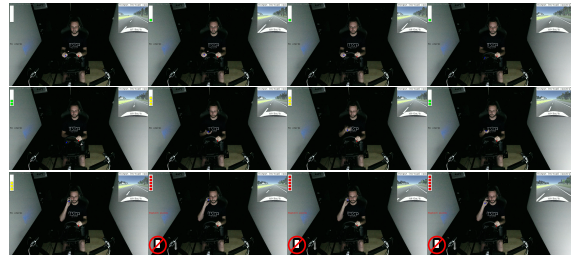
Figure 5: The sample sequence of output of the sg5#s140, where the buffer of the lasts 5 predictions for risk is shown at the top left, and the indication of the output alarm is on center left (black text indicates no alarm, yellow is lowest alarm, red is highest alarm).
