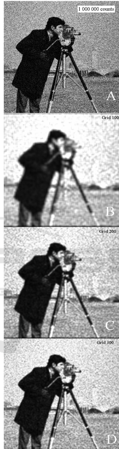
Figure 3: Reconstructions of “cameraman” image (1 000 000 counts) by various number of components K in intermediate representation: A – the original image in TIF format, B, C, D –reconstructions, corresponding to K = 100^2, 250^2, 300^2 components.
