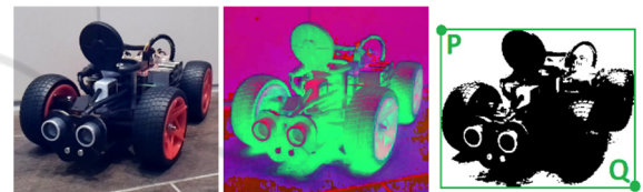
Figure 2: Automatic annotation with the HSV colour space. Left: Model car in RGB format. Middle: Model car in HSV format. Right: Model car as binary image with founded coordinates for P and Q.
