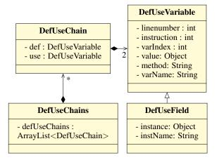
Figure 1: An overview of the DUCs implementation. Methods are omitted for the sake of clarity.
