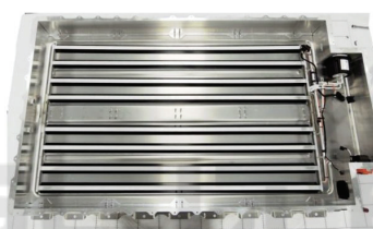
Figure 21: BMW i3 bottom refrigerant cooling plate layout (Munro, 2020).
