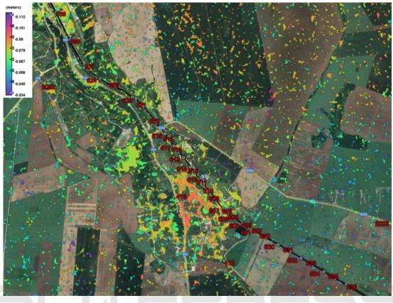
Figure 4: Subset of displacement map for the period Oct 2018-10 March 2019 and geodetic points from railway route.
