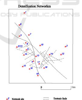
Figure 2: The geodynamic network for the area of the Mirovo salt deposit - general scheme (Valev et. al., 2015).
