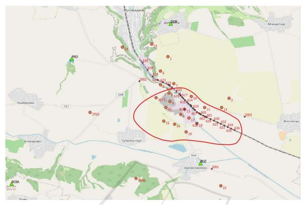
Figure 1: Local seismological network (green triangles), local geodetic network (red dots) and local geodetic network for railway monitoring (red stars) in the area of the Mirovo salt deposit (red contour).
