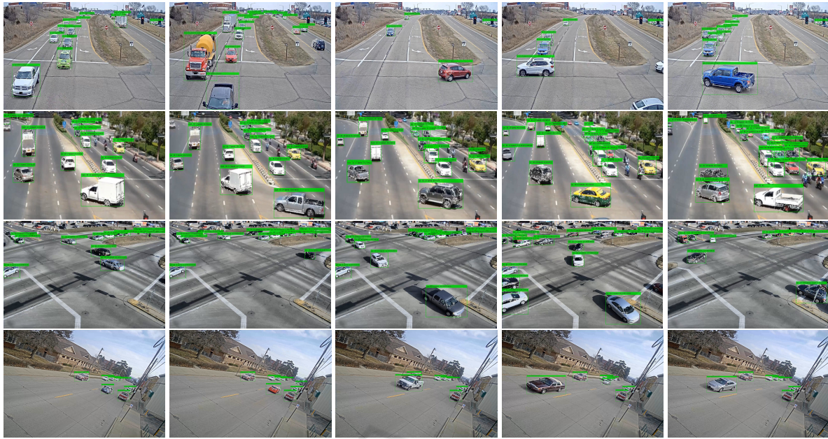
Figure 2: Output of proposed algorithm. Speed estimations of a number of vehicles with various sizes moving into different directions validate the effectiveness of our proposed algorithm. Videos from different data sets have been used in this set of experiments.
