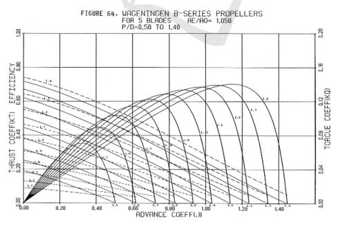
Figure 2: Performance curves of the propeller.
