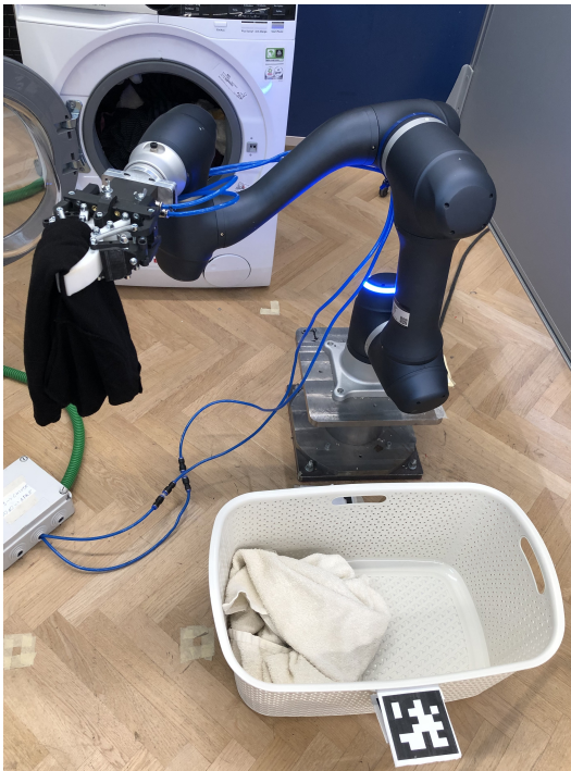
Robot successfully grasped an item from a laundry basket and midway to place it inside the washing machine.
