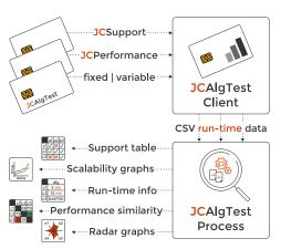
Figure 1: A high-level overview of the components and processes of our audit suite. The on-card applets measures the specification compliance and benchmarks the performance. Then, the client collects and processes the results to extract a useful information.
