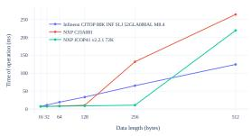
Figure 2: The example relationship between the input length with the runtime of 3DES with ISO9797 M1 padding in three different commercial JavaCards. The nonlinear increase for NXP CJ3A081 card between data with 128 and 256 bytes can be explained by memory limits of internal processing buffers, providing information about the hardware used.
