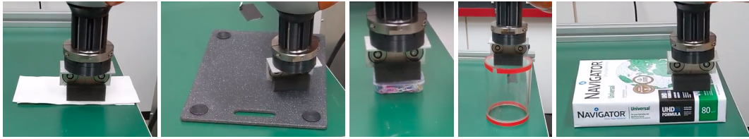
Figure 8: Single point configuration for different objects: a) Tissue. b) Board. c) Small box. d) Hollow cylinder. e) Paper bundle.
