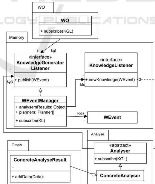
Figure 5: Static model of Monitor, Analysis & Knowledge.
