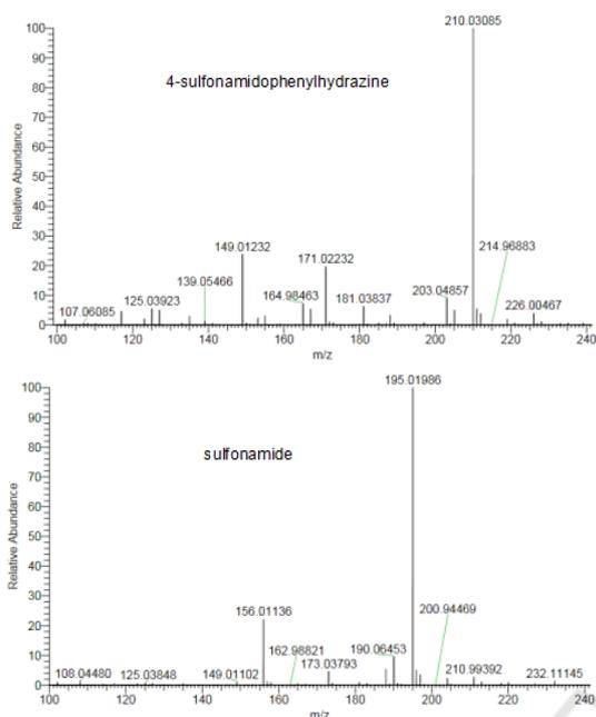
Figure 1: Representative mass spectra of 4-sulfonamidophenylhydrazine and sulfonamide.
